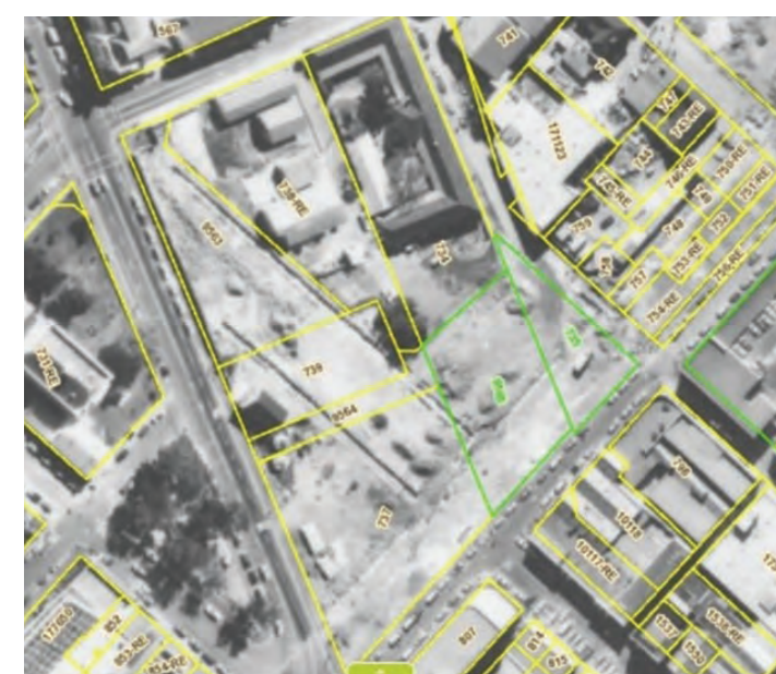
Figure 4. 1981 aerial photo showing construction on the new Somerset Road alignment and widening of Buitengracht Street. St Stephens church and the Salvation Army/Workman's Metropole building have been demolished. (Source: CoCT map viewer in Halkett, 2024)
