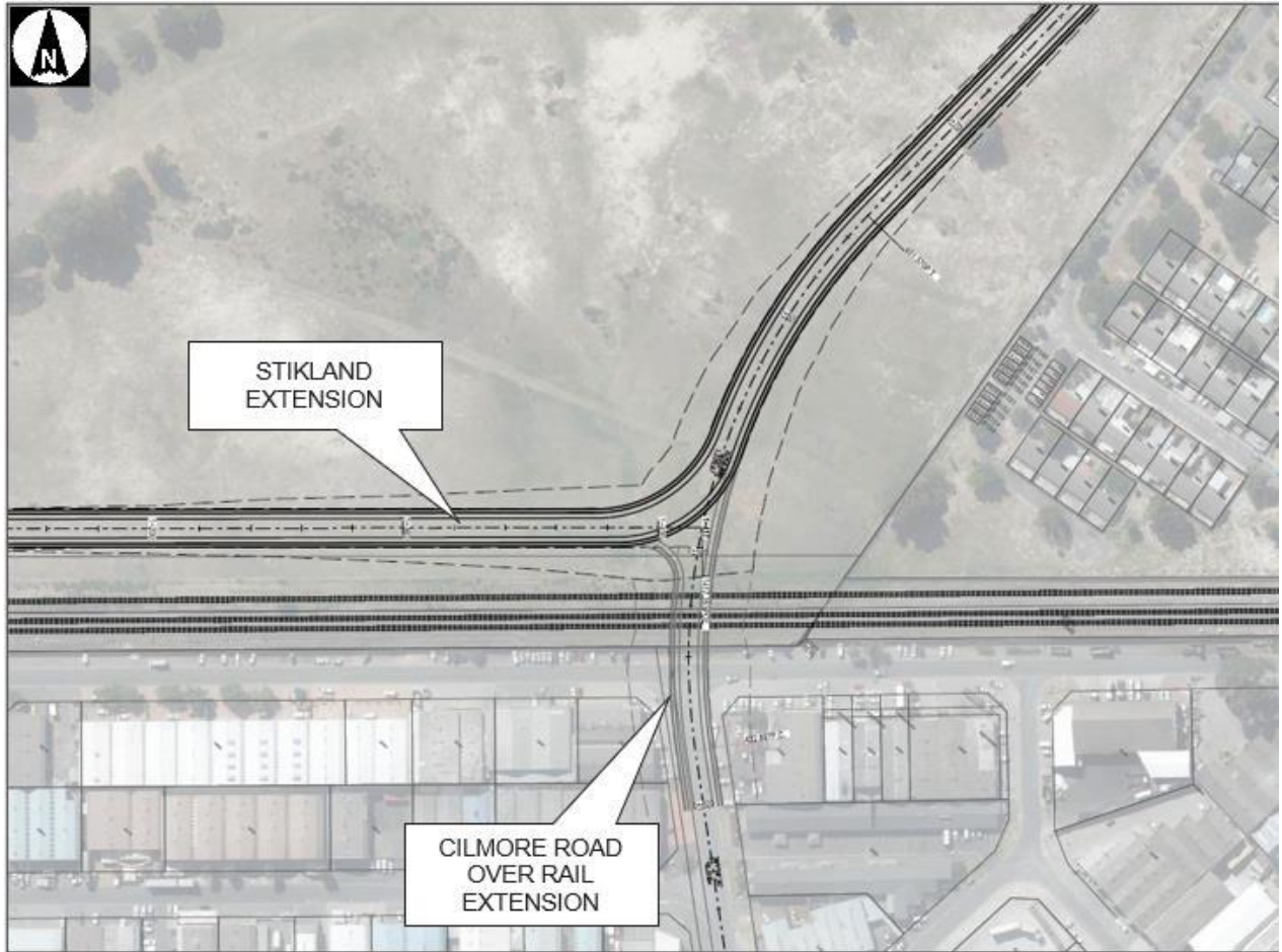
Figure 7.2-3 Concept layout of Stikland extension and Climore Street Road over rail crossing (Source Bellville Future City Report)
