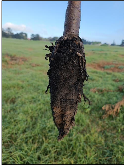
Figure 7.9-9 Soil auger sample taken within the area of dense kikuyu grass indicative of wetland conditions. Note the dark, organically rich surface component overlaying lighter reddish soils indicative of elevated levels of clay.
