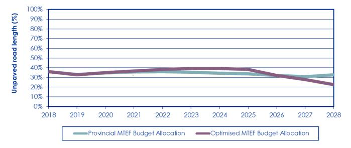
Figure 5-38: Predicted proportion of maintained unpaved roads with possible passibility problems where gravel thickness is <50 mm
