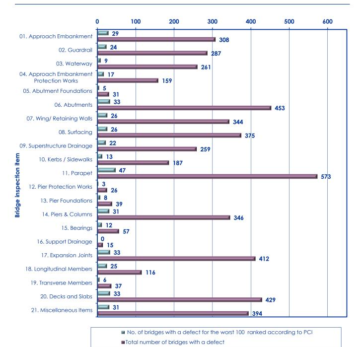
Figure 4-13: Statistics for the defects on bridges
