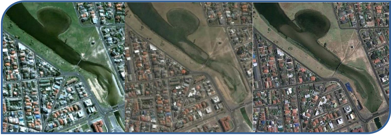
Figure 5: Images from Google Earth showing the migration of the sandflats upstream from the mouth and up the Narrows. The Royal Road bridge can be seen in the lower right corner of each image (after Killick).
