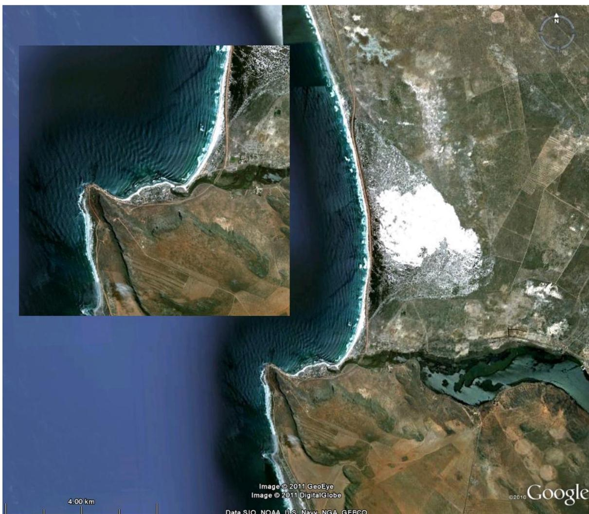
**Figure 2-3** Log spiral bay development at Elands Bay. Inset shows wave refraction around Baboon Point.
