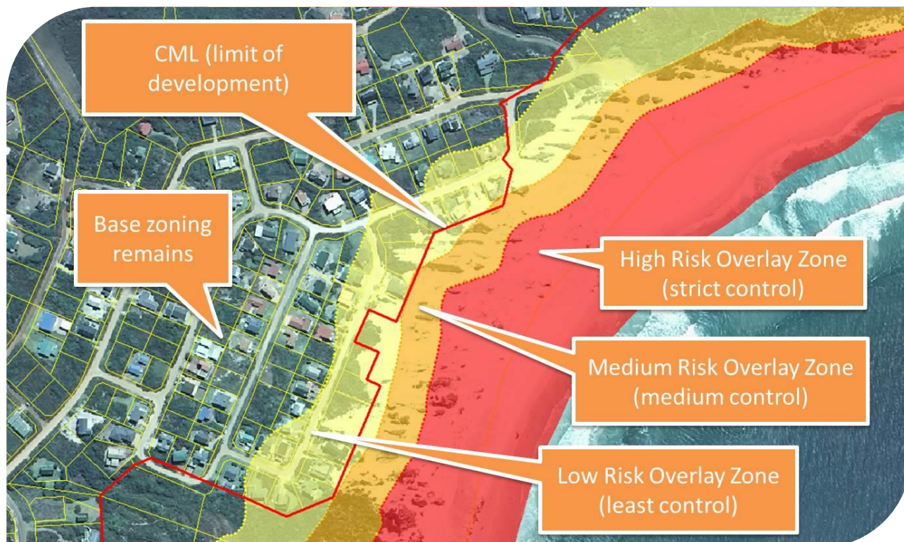
Figure 15: Example of the combined coastal management (set-back) line and overlay zones (urban or developed area)
