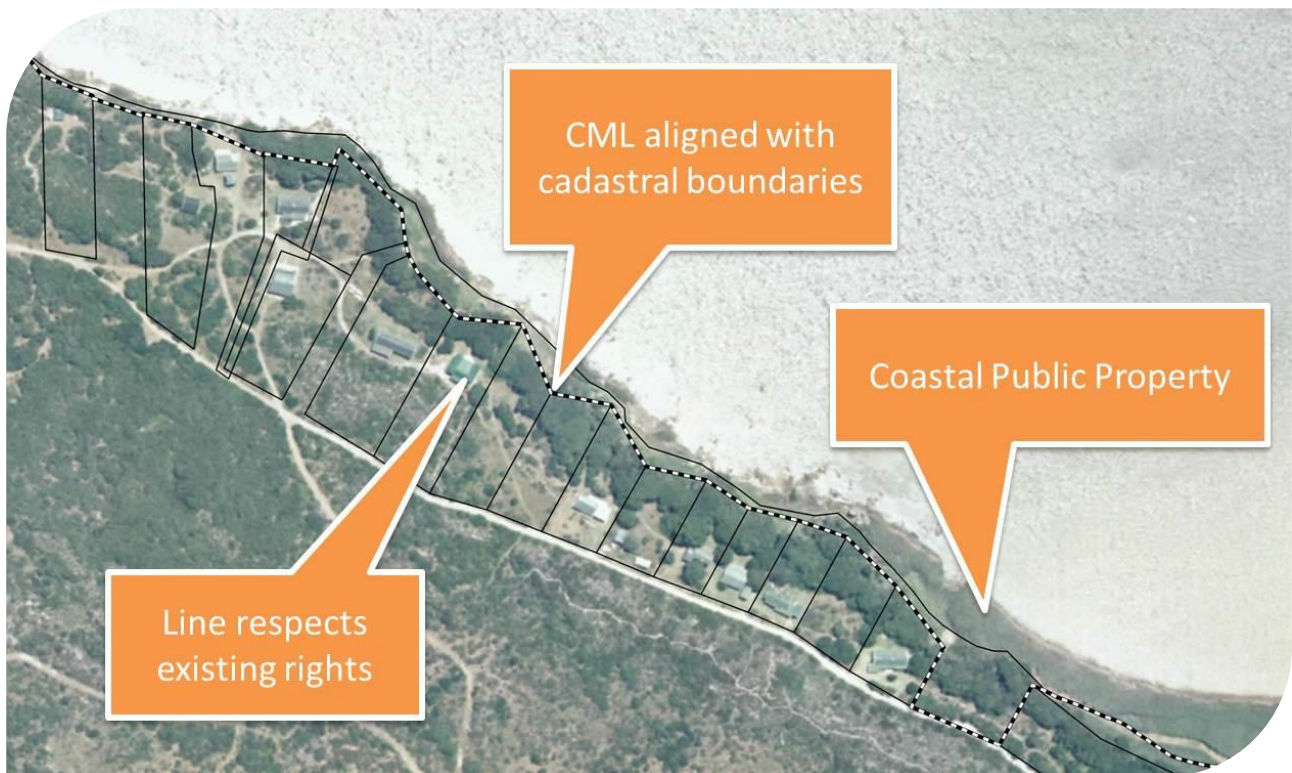
Figure 11: Example of the location of the coastal management (set-back) line in developed parts of estuaries
