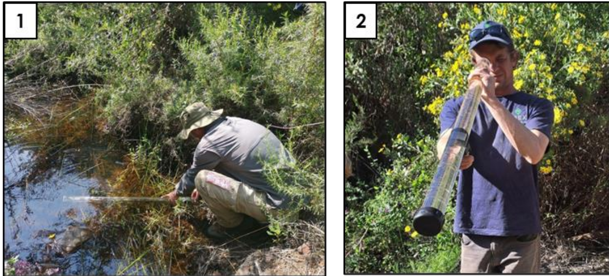
Figure 26: (1) Collecting water in the water clarity tube; and (2) determining the disappearance and reappearance depths.
