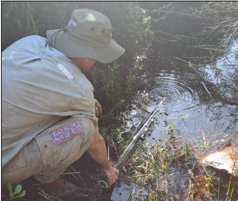
Figure 24: Water being collected in a clarity tube within a stream.
