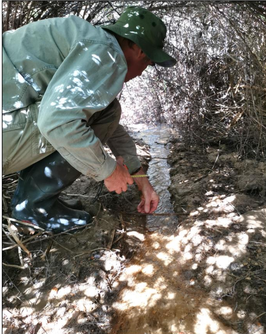
Figure 40: Testing out the float method at Site 3.
