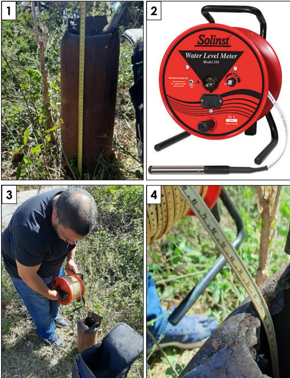
Figure 20: Summary of the Borehole Water Level Dipmeter method: (1) measuring the height of the borehole above ground, (2) a water level dipmeter, (3) taking the water level measurement in the borehole, and (4) ensuring that the dipmeter is measured at the same point consistently. (Images: Solinst, 2013.; Petersen and Strydom, n.d.).
