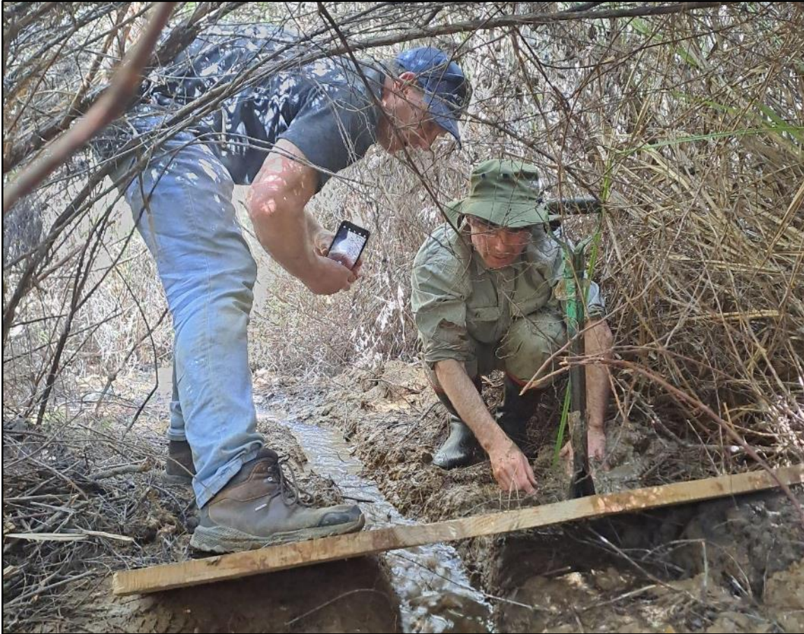
Figure 7: Size of streams for which the V-notch weir method is ideal (Image: ACS, 2023).
