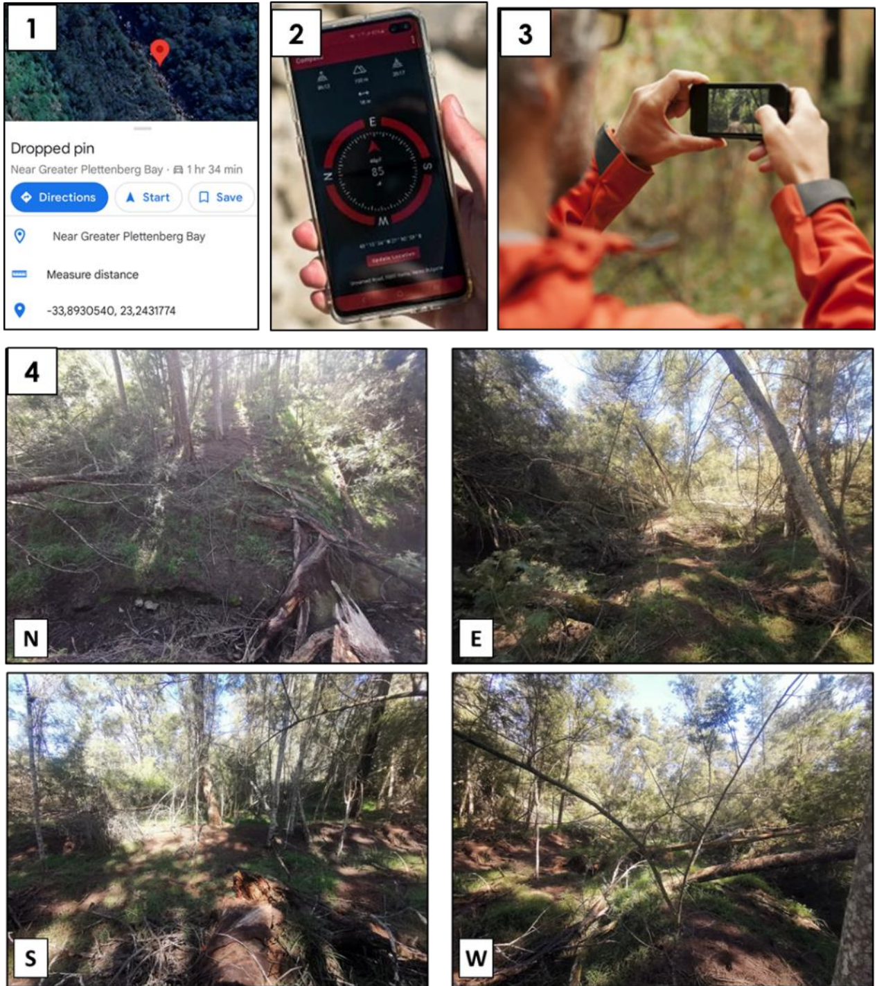
Figure 35: Summary of the Fixed-point photography: (1) Record location, dropping a pin. (2) Use a compass or compass application to find each direction (North, South, East, West). (3) Take a photograph at breast height. Take a photograph in each direction (N- North; S- South; E- East; and W- West) (4) (Images: ACS, 2023; phonearena, 2023; active, 2013).
