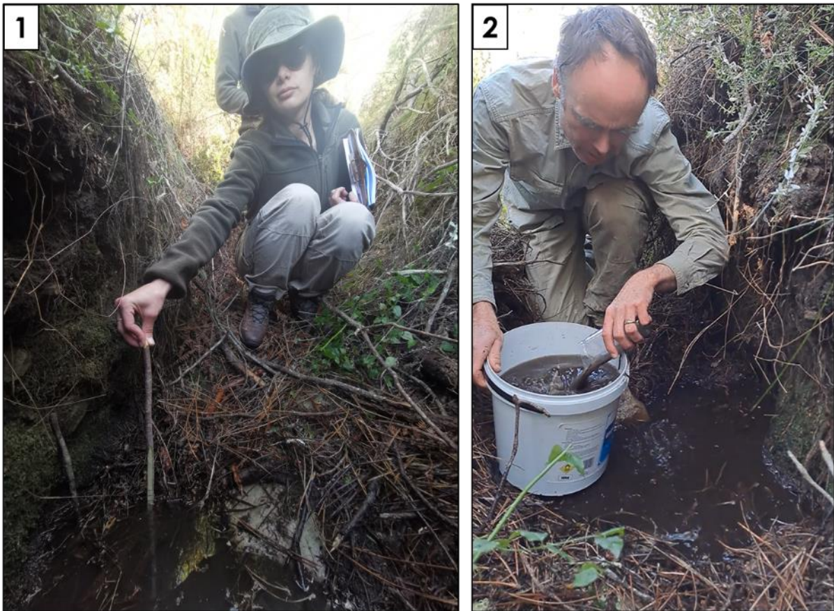
Figure 18: The spring discharge water recovery method: (1) the water level in the depression is measured and marked on a guiding stick; and (2) a container of known volume is then used to remove water, and the time taken for the spring to refill the depression to the previously measured water level is recorded.
