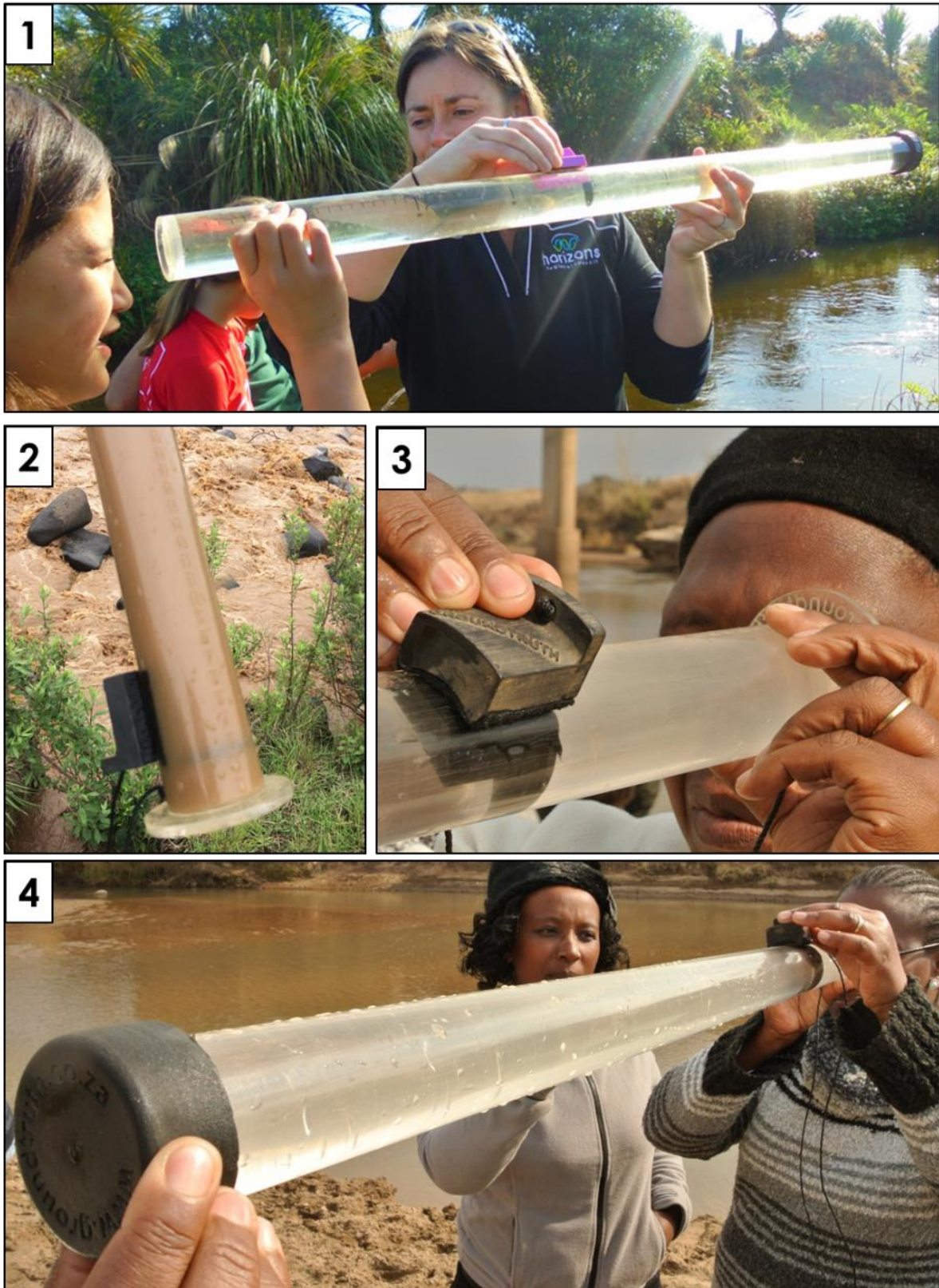
Figure 25: The (1) water clarity tube with its different components: (2) base through which the target is viewed; (3) the magnets which are shifted to move the target; (4) and the stopper sealing the bottom of the tube (Images: Nzaae, n.d.; Ground Truth, n.d.).
