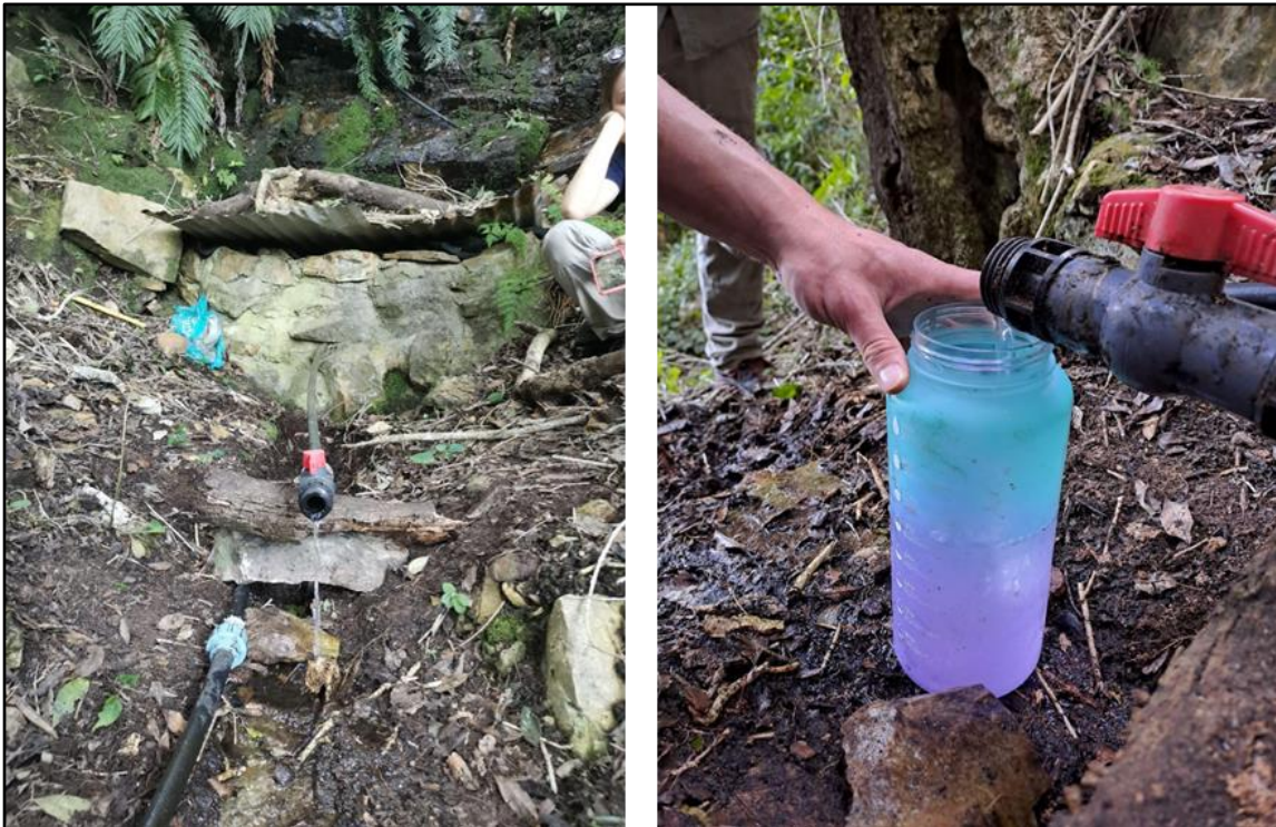
Figure 16: Collecting spring discharge from a single output in a container for the container fill method (Images: ACS, 2023).
