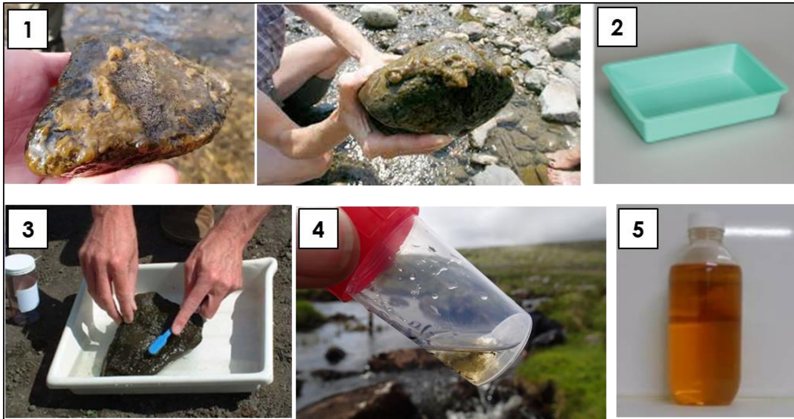
Figure 30: Summary of using the diatom method: (1) Collect substratum; (2) rinse rocks and place in tray; (3) collect diatoms from substratum; (4) deposit diatoms to sample bottle; and (5) preserve and store samples (Images: Kelly, 2015; National Geographic, n.d.; Franchini, 2013; Kelly and Yallop, n.d.; Kelly, 2022).
