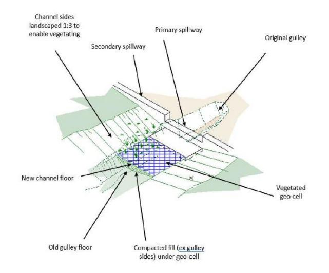
A view of a weir in a gulley showing the original gulley, landscaping, the geo-cell, and the compacted fill lifting the floor of the old gulley
