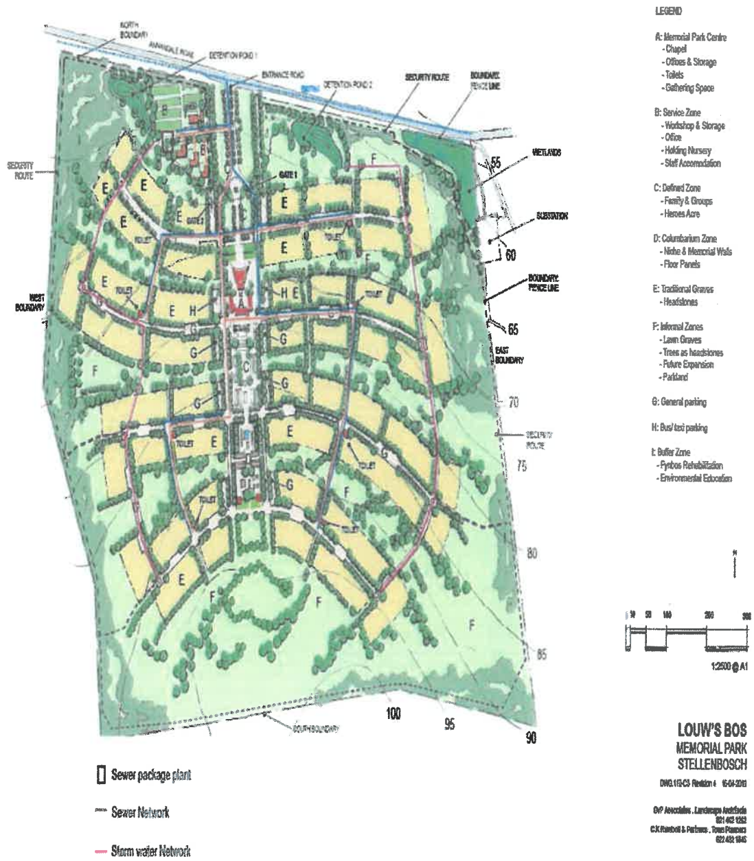
Figure 3: Storm water and sewage plan layout.
