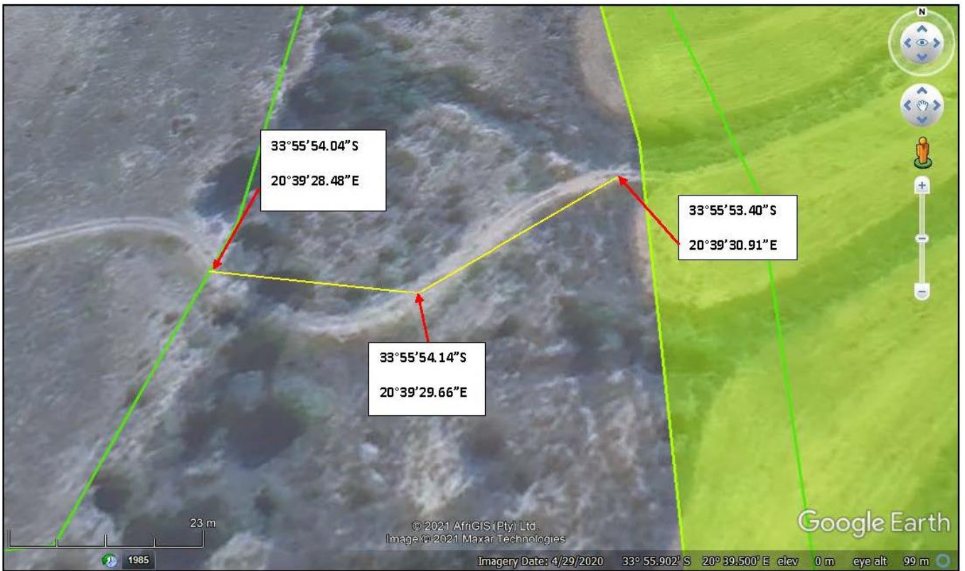
Figure 1: Yellow line with coordinates indicating new pipeline section over river crossing (total length 72.3m)
