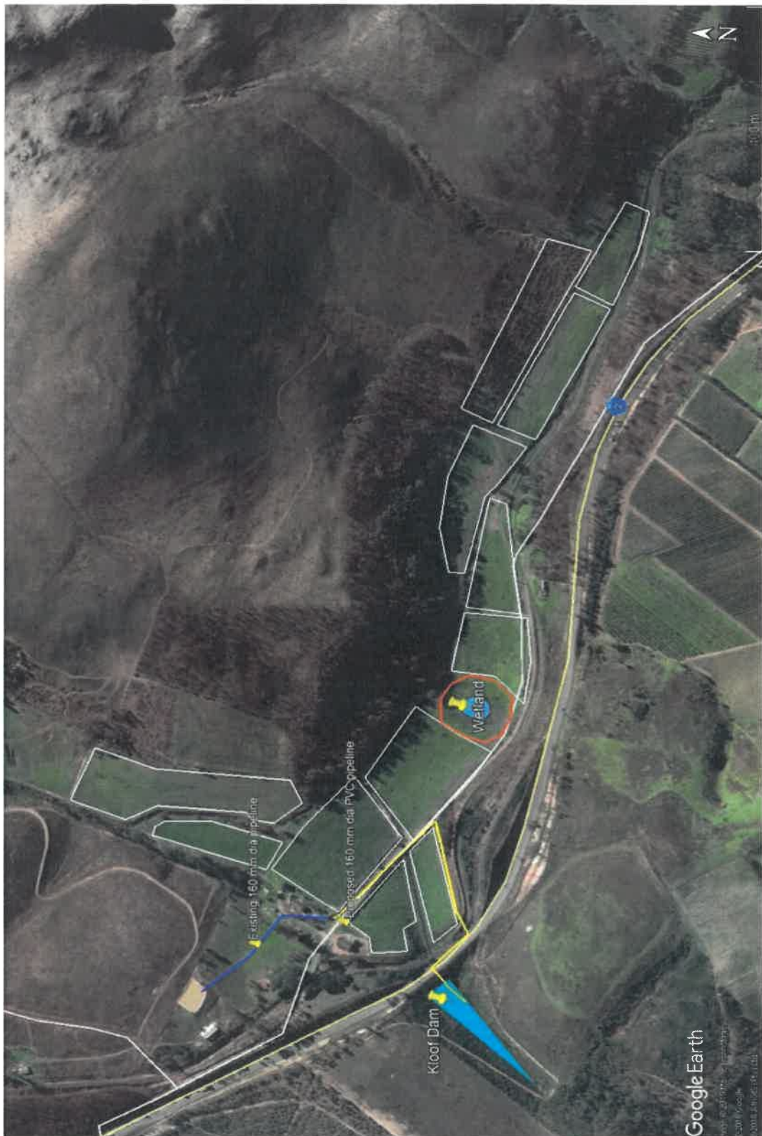
Figure 2: Site Layout Plan depicting the preferred alternative (herewith authorised) which includes the delineated wetland buffer area, 17ha of cultivation area blocks, the Kloof Dam and the construction of a new 160 mm diameter PVC pipeline (0.6 km length) from the existing pump house to the new Kloof Dam.
