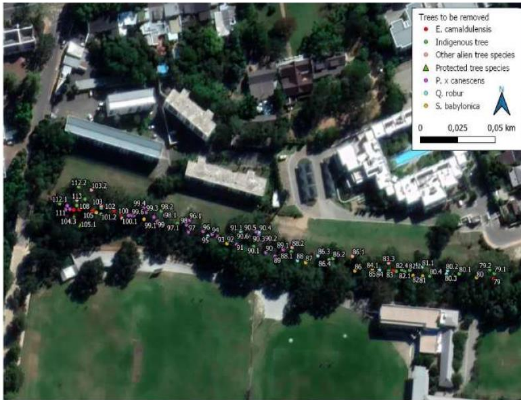
Figure 5: A map of the Eerste River between Krige Street and Aan De Wagen Weg showing all the trees that need to be removed to allow for the pulling back of the northern banks to reduce the slope.
