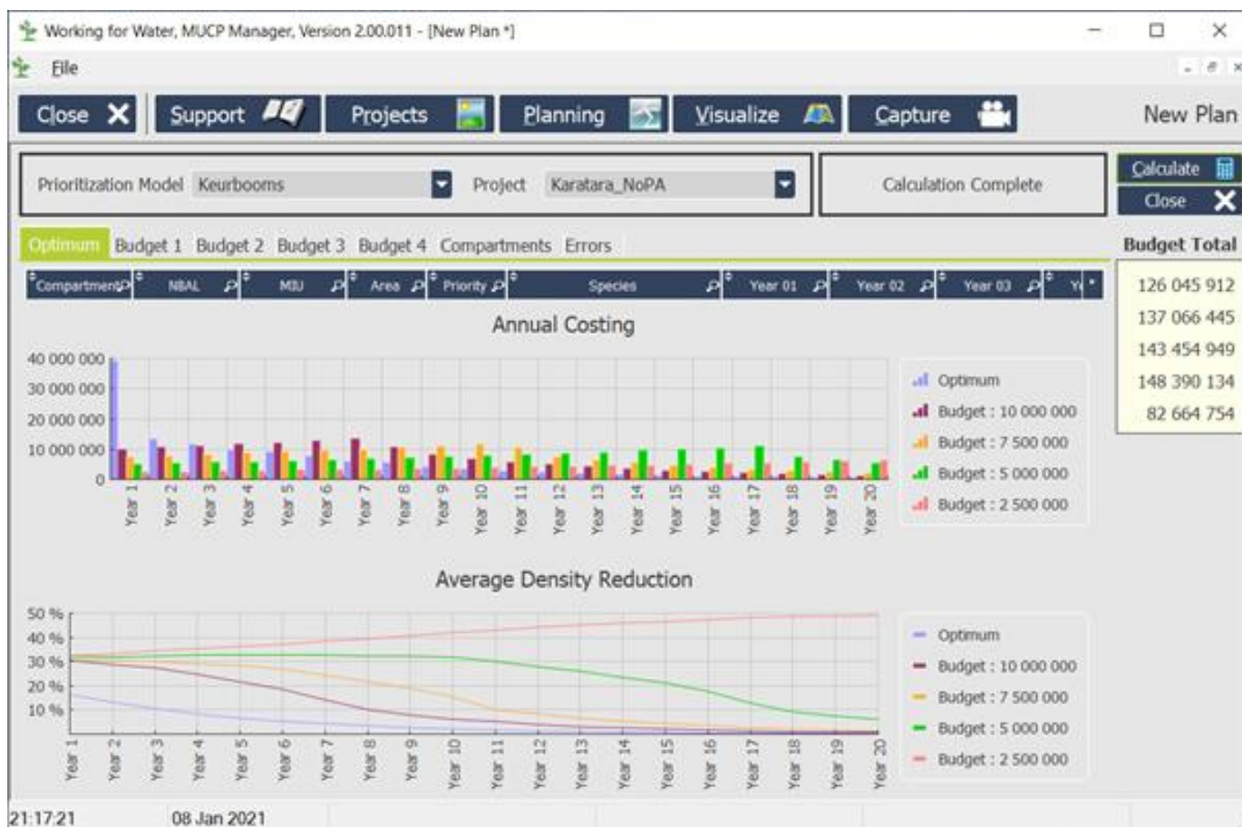
Figure 2 MUCP manager extract. Projected density reduction based on AIP clearing budget scenarios over a 20-year period.
