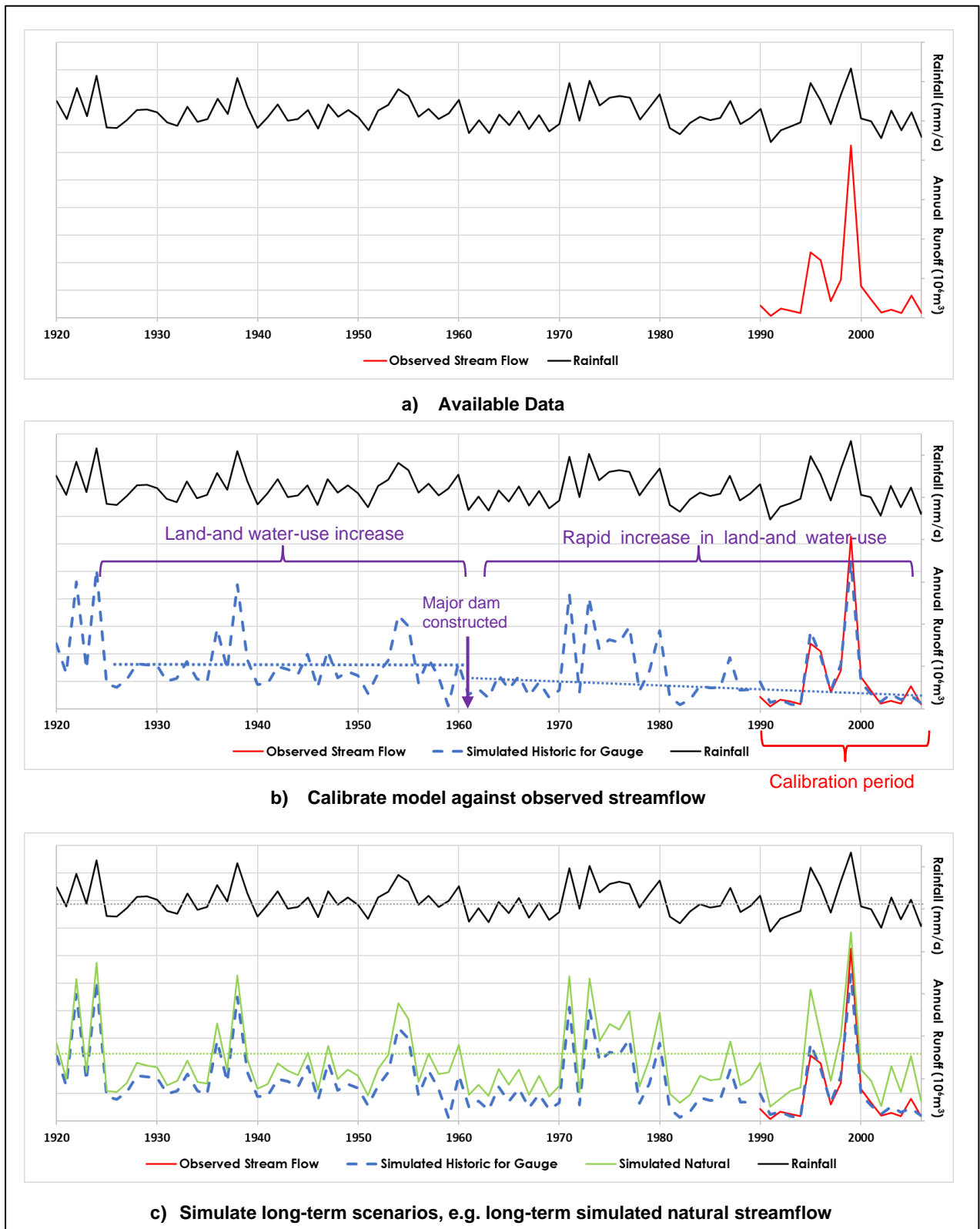
Figure 13: An example to illustrate the purpose of rainfall-runoff modelling, model calibration and scenario based simulated hydrology.
