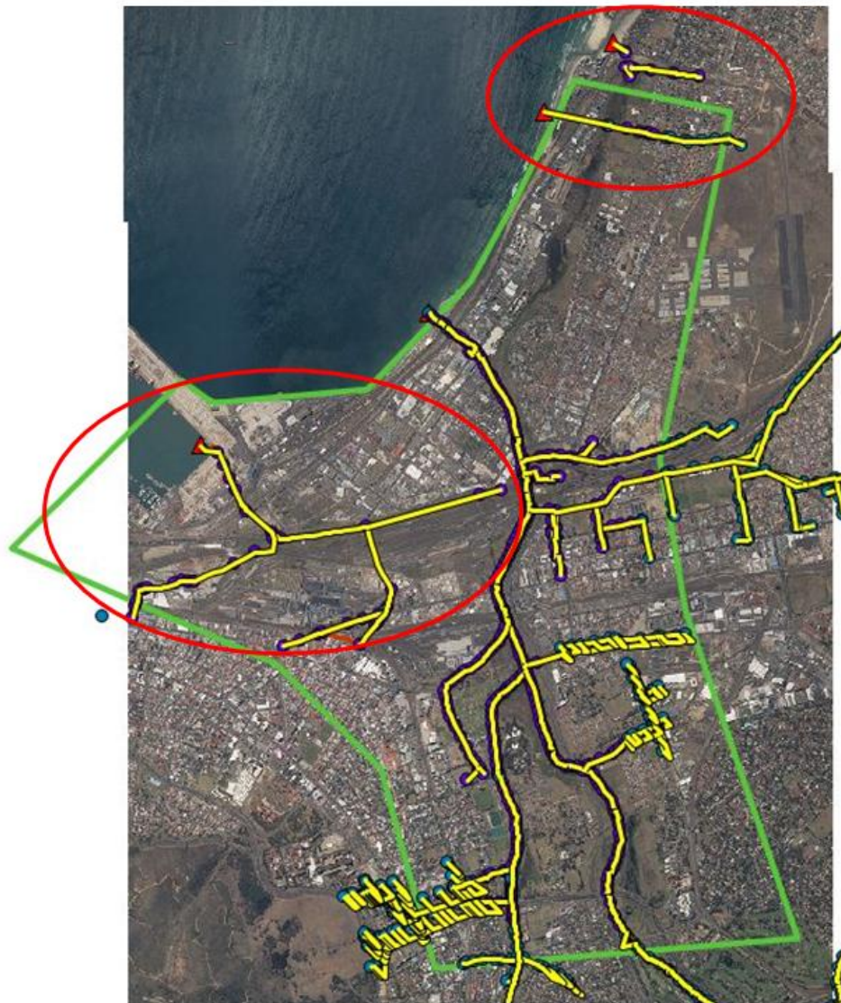
Figure 10: Modelled areas of the bulk stormwater network outside the Salt River catchment
