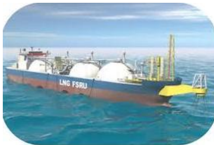
Figure 3-2: Turret Moored FSRU
