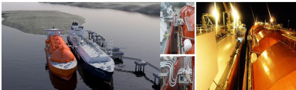
Figure 4-3: Side by side operating FSRU moored at a Jetty (Hoegh LNG website)
