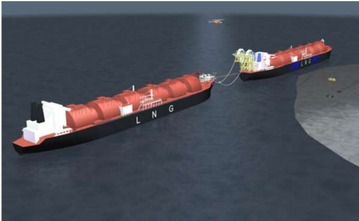
Figure 2.4 LNG transfer from a supply vessel (on the left) to a FSRU (on the right), using the tandem system (Golar Bluewater, 2011)
