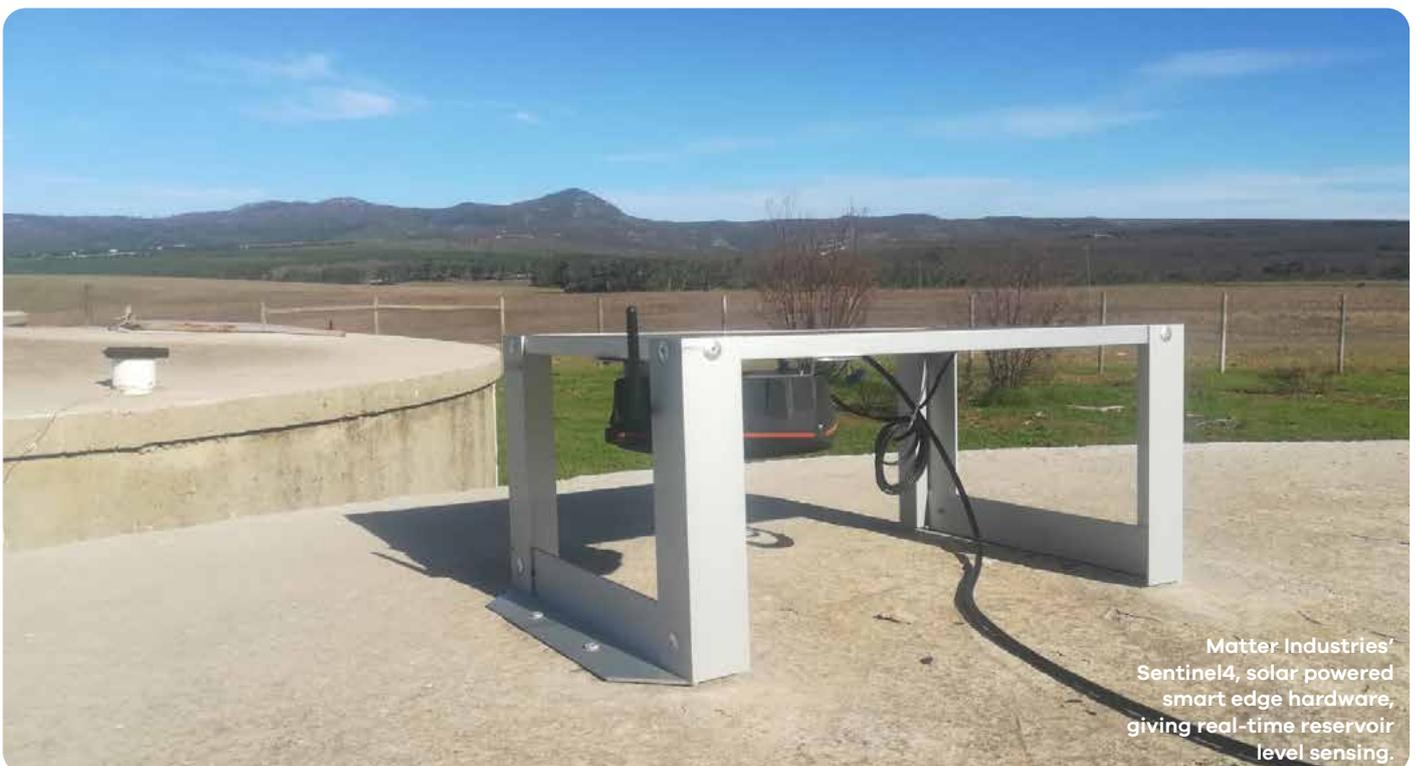
Matter Industries' Sentinel4, solar powered smart edge hardware, giving real-time reservoir level sensing.
