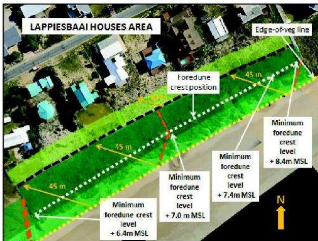
Figure 17: Position of the recommended minimum crest height
