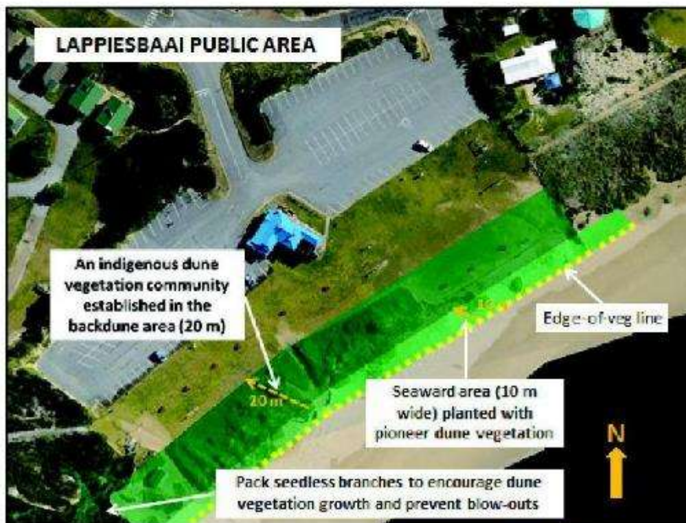
Figure 11: Details of the vegetated areas within the buffer dune
